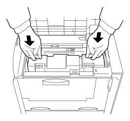
**6.** After the toner container is installed, set the two toner container release levers to the left position (fixed).
